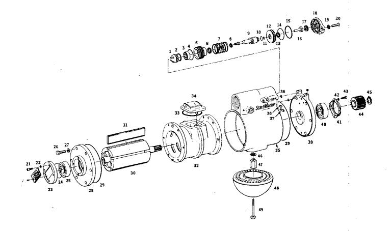
STARTMASTER SERIES 250 AIR MOTOR FOLD-OUT NO. 4
