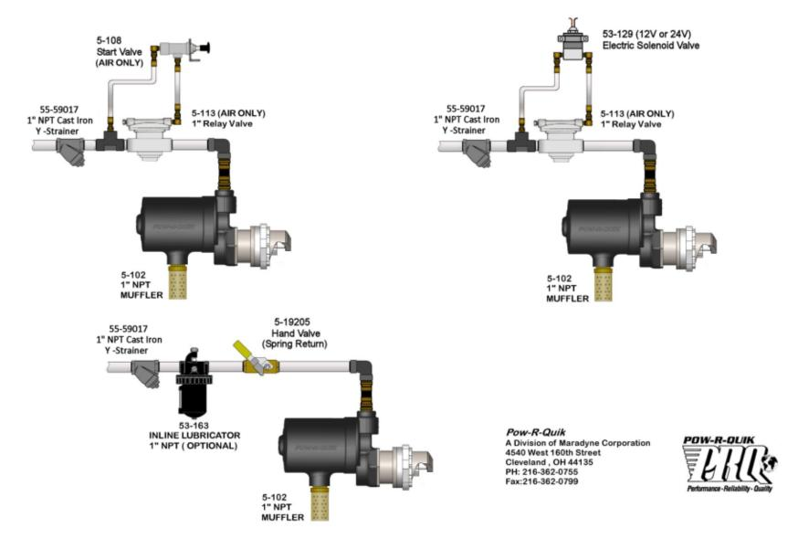
WARNING: Penetrating oil attack rotor vanes and cause motor failure. USE DIESEL FUEL OR SAE#10 NON-DETERGENT LUBE OIL ONLY.
